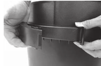
Step 1 Remove the protective cap and then open the large clamp on the canister.
