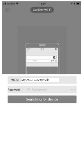
10. Fill in the password for your Wi-Fi network (selected by your Wi-Fi setting in your mobile phone). Press "Search".
